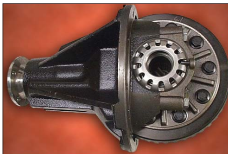
Spiralock thread forms are used by Dana Corp. to fasten the ring gear shown above to the driveline of axles.
